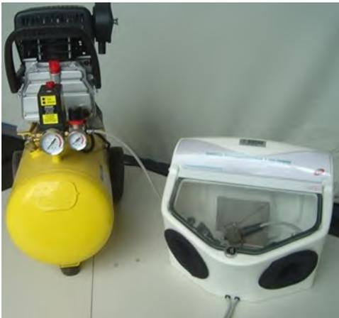
Figure 1: Blasting chamber and compressor.
