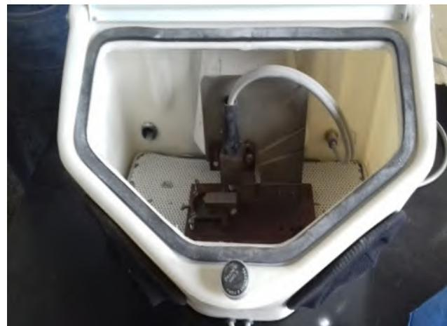
Figure 1. Blasting chamber with the support inside
