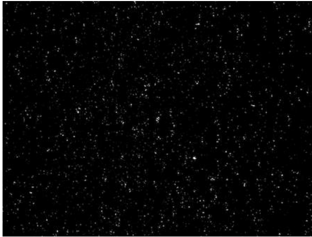
Figure 2: Same image in Figure 1, but after digital processing to identify and quantify the presence of pores.
